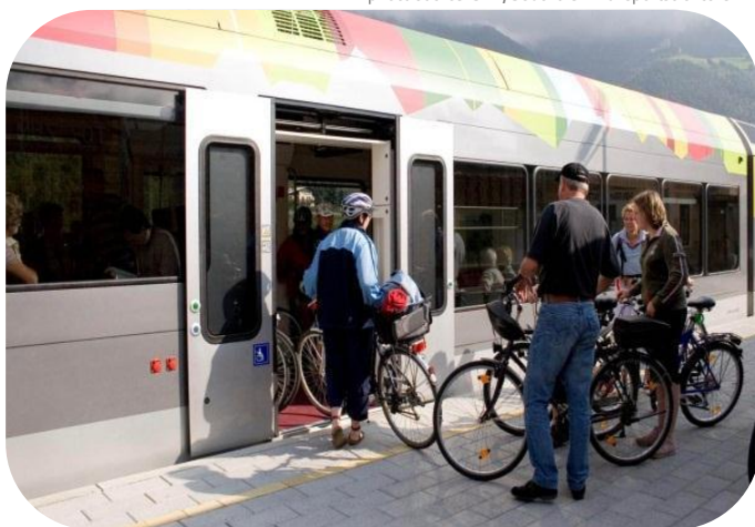
Low floor wagons for barrier-free access photo source: STA, Südtiroler Transportstrukturen AG
