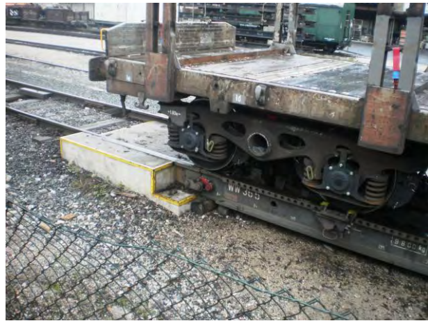
Transport of standard gauge wagons on special units ("Rollwagen" ) of the narrow gauge and rolling down to the normal gauge rails, photos: Ernst Lung
