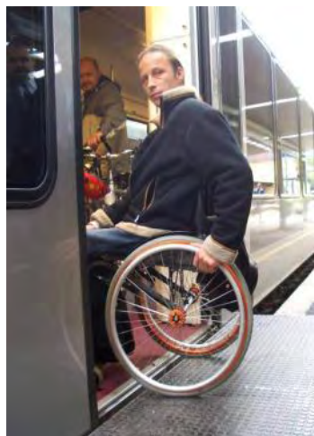
Low floor train units and entrances without stairs, photos: STA
