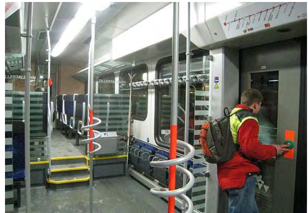
low floor section with multi-purpose space to transport luggage and bicycles Photo: Otfried Knoll
