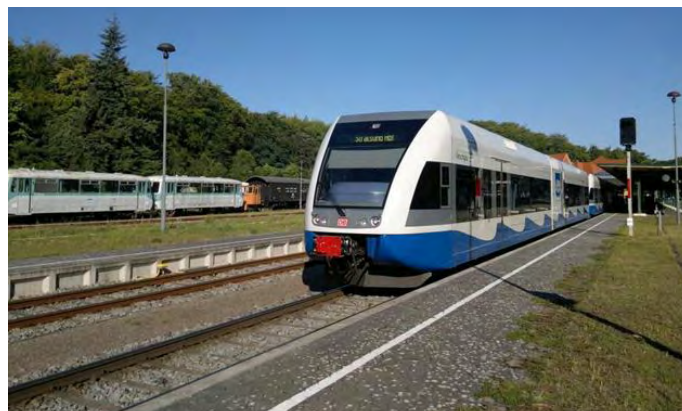
New low floor train GTW 2/6 and old train units ("Schienenbusse"), photo: Otfried Knoll
