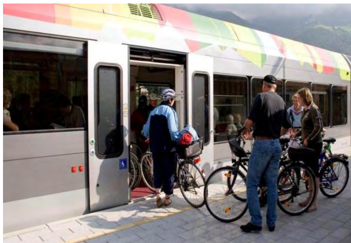
Low floor train units and entrances without stairs, photos: STA
