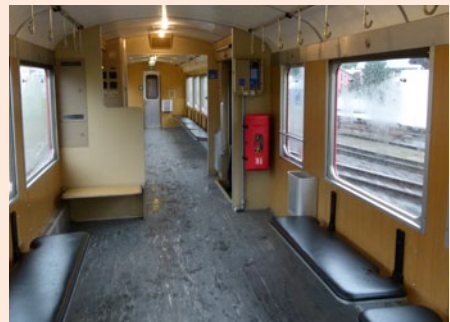
A passengers wagon of the Rhaetische Bahn was converted to an easily accessible and spacious bike wagon
